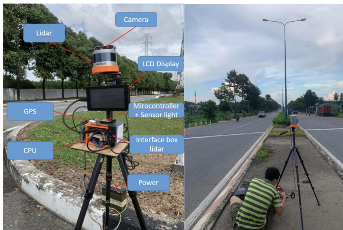
Fig. 8. Roadside system setup in the field test (left), setting lidar at the middle of the lane (right)
